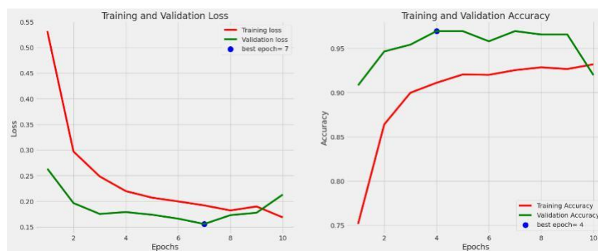
Image 2: Graph of the epoch and loss progression to achieve the best accuracy for the 2-layer convolution CNN architecture on the imbalance dataset
